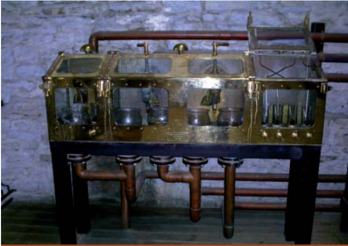
The stillman tests the strength of the spirit in the Spirit Safe
