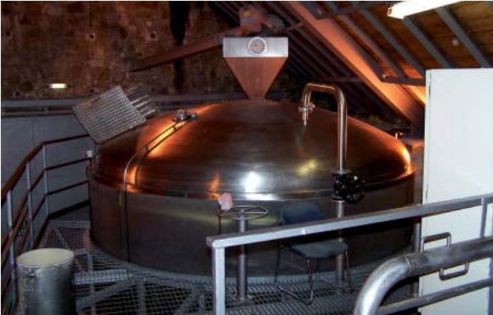
It is then steeped in the mash tun (“the coffee filter”)
